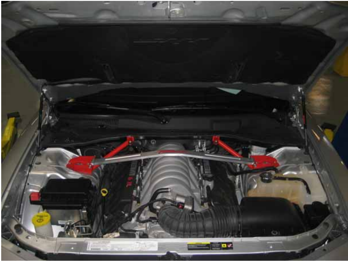
Image 9: Techco Strut Tower Cross Link Brace on Dodge Charger SRT8
