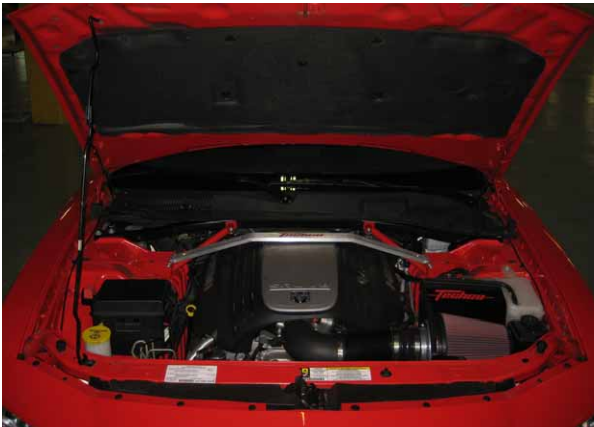
Image 10: Techco Strut Tower Cross Link Brace on Dodge Charger R/T
